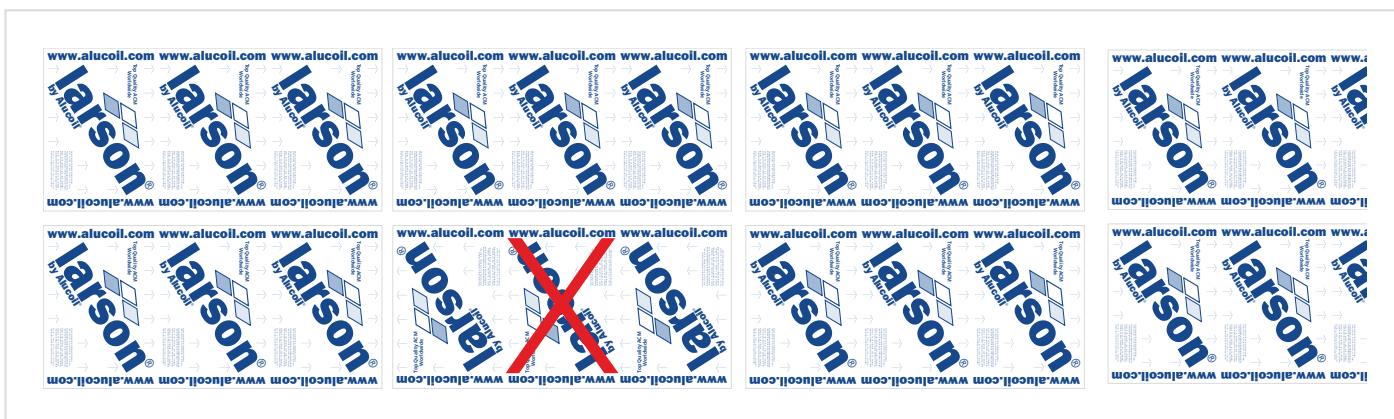
Importance of the direction of the arrows in the placement of metallic colors
