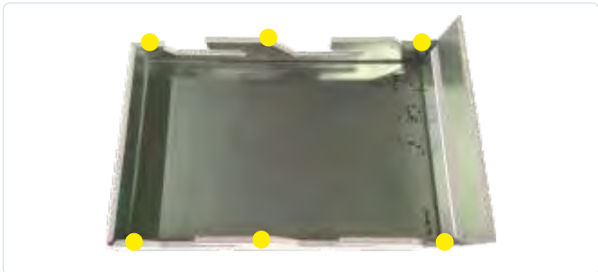
3. Folding the lateral edges and the triangular parts of the cassette to 90°.
