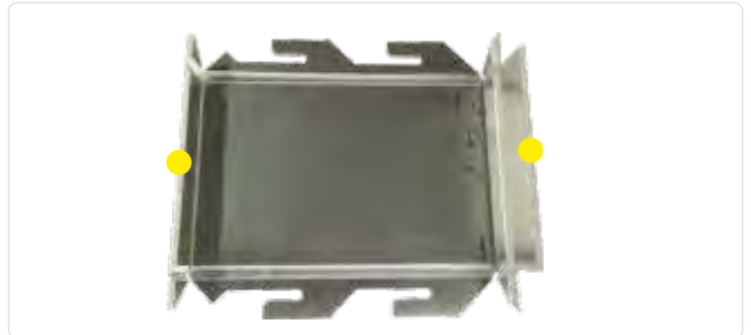
2. Folding the upper and the bottom edges of the cassettes to 90°.
